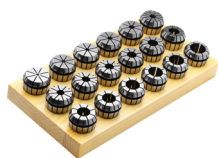
Collets set with cooling channels in wooden sockets DIN 6499 A (ISO 15488 A) ER-system with square locking drive for tapping drills
